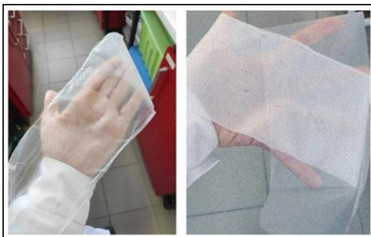
Figure 1. PHB membranes produced through bacterial synthesis ( Burkholderia sacchari DSM 17165).
