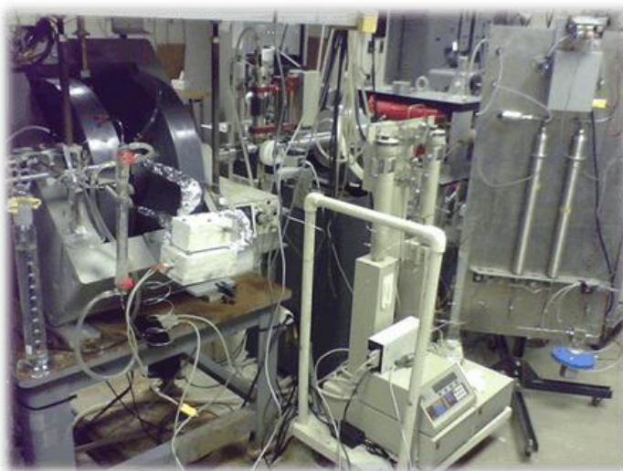
Figure 1. High Pressure/Temperature EPR apparatus at Notre Dame Radiation laboratory 3MeV van de Graaff accelerator.
