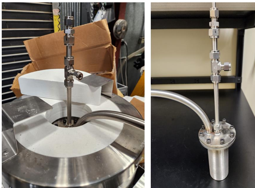
Figure 6. (left) High-temperature nebulizer staged in the furnace planned for initial testing. (right) The high-temperature nebulizer for initial tests.
