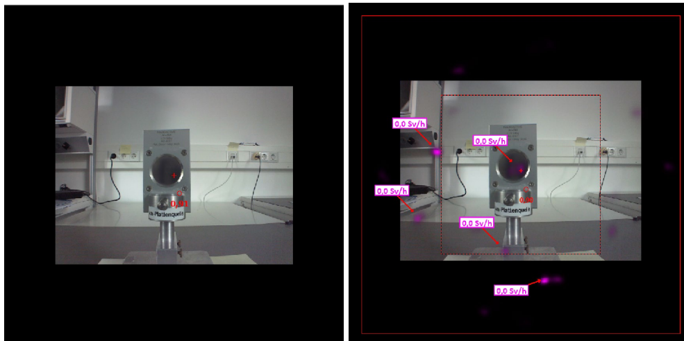
Figure 5: ^{241}\text{Am} source for 310 s in a distance of 30 cm. Left: Compton image. Right: Coded Mask image. The position of the source is not detected.
