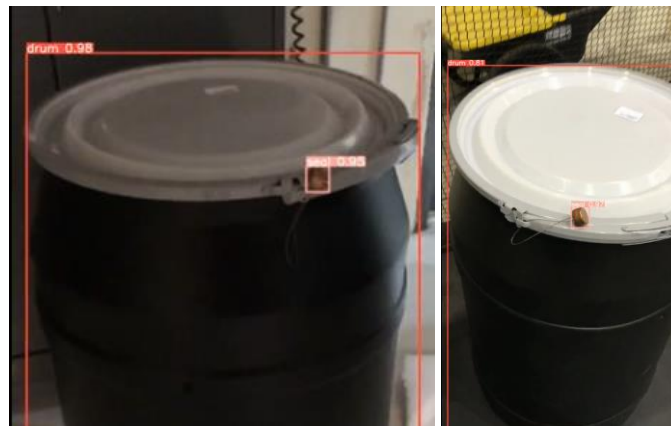
Figure 5: Test results for object detection of 55-gallon drums and metal cup seals, with confidence level displayed.
