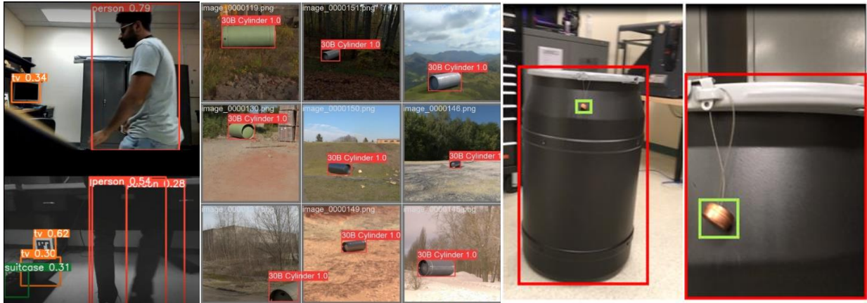
Figure 4: Progression of object detection training. (Left) COCO dataset for common objects, (Center) Limbo dataset for UF 6 and other cylinders, (Right) 55-gallon drums and metal cup seals at the AutonomyNM testbed.
