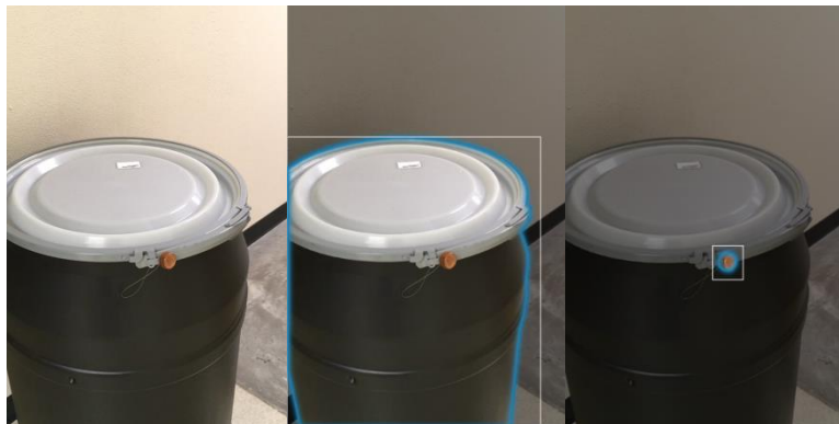
Figure 8. SAM segmentation from bounding boxes for drums and seals.
