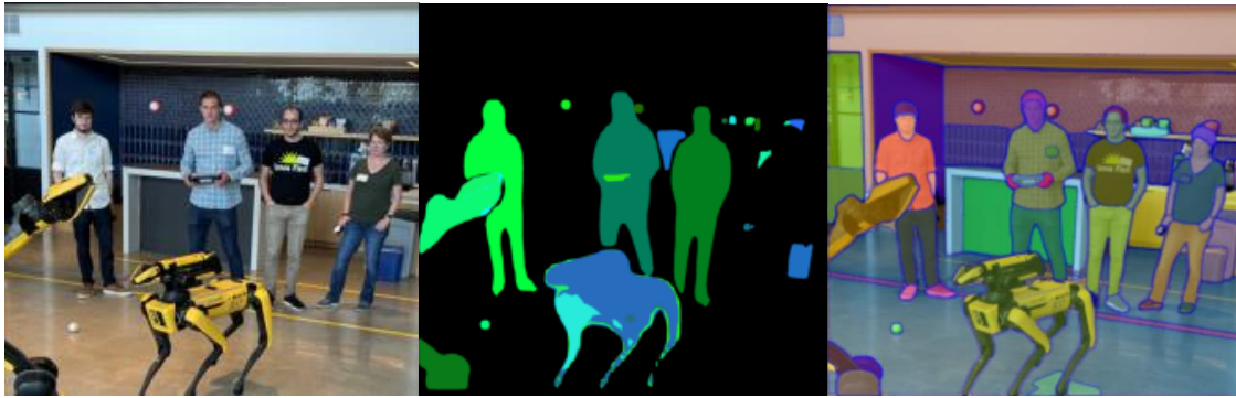
Figure 7. Pretrained segmentation results. Mask-RCNN in the middle. Segment Anything Model on the right.
