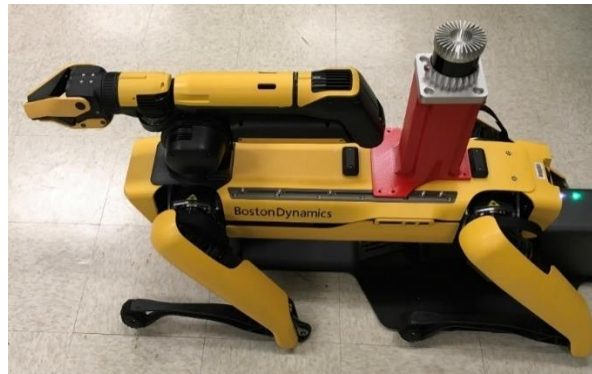
Figure 10: Spot with Ouster OS1 LiDAR payload.
