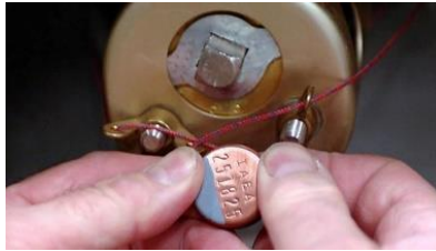
Figure 1: CAPS metal seal, image: IAEA, 2020.
