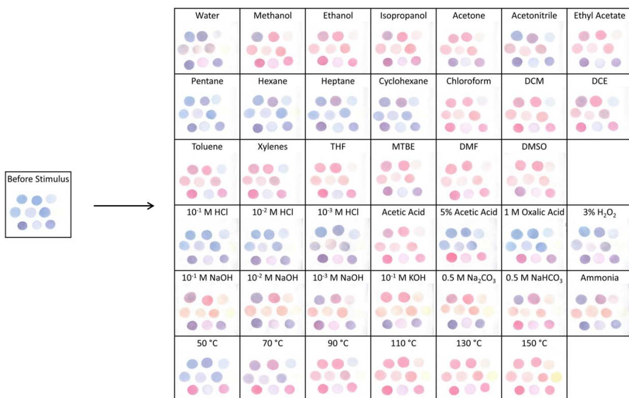
Figure 4. Paper-based PDA arrays before (left) and after (right) stimulus exposures. The order of PDA sensing spots matches Figure 3: top row, left-to-right: PCDA, TCDA, DCDA; middle row, left-to right: PCDA+DCDA, TCDA+DCDA, PCDA+TCDA+DCDA, DPHD; bottom row, left-to-right: EAE-PCDA, EAE-PCDA-Br, EAE-PCDA+EAE-PCDA-Br.
